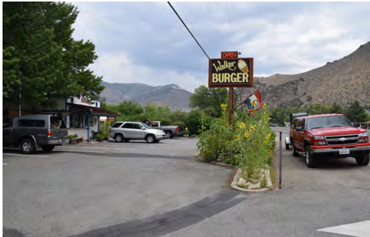
A slip lane is a type of business frontage that provides access to parking off of the high-speed highway; it can be seen above at Walker Burger.
