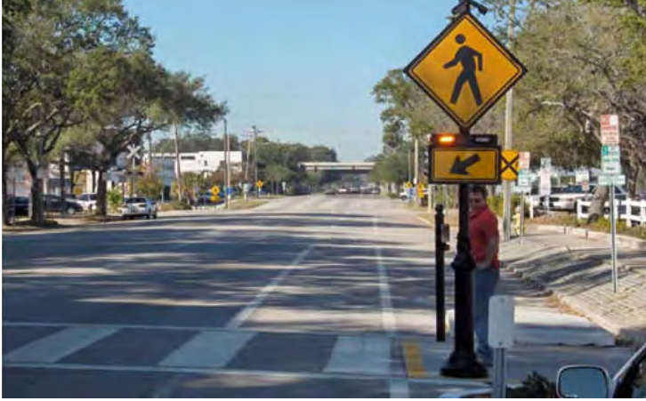
Rectangular Rapid Flashing Beacon flashes every second to announce that a pedestrian is present at the roadway. Photo credit: http://mutcd.fhwa.dot.gov/resources
